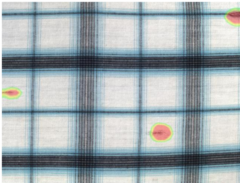
An example of textile defect detection using the DL_DetectAnomalies2 .
